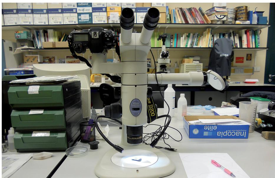
**Figura 2.** Lupa binocular
