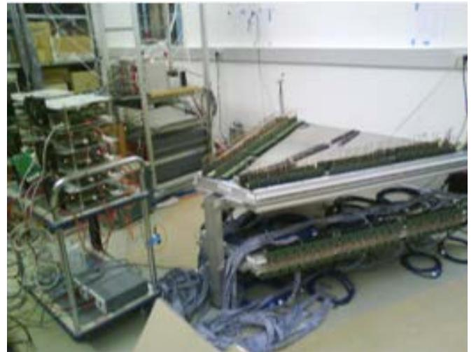
Fig. 5 - Setup for taking cosmic ray data with couples of RPC detectors of the HADES low angles TOF wall at the GSI (Darmstadt). A. Blanco et al. (2012).
