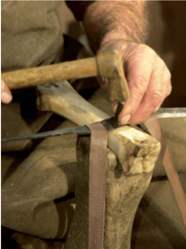
Fig. 6. Blacksmith pinking the sickle using a bone anvil. Photograph taken from Esteban and Carbonell (2004).
